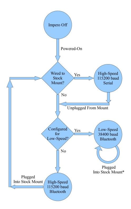
\*A stock mount communicates at 115200 baud, and the Impero will not recognize it in this situation.
